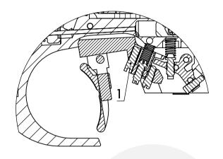
PLEASE NOTE: Too fine adjustment of the trigger stop may cause inconsistent trigger weight and release.
