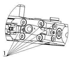
ATTENTION: At maximum offset of the grip, please ensure that the grip does not press against the pistol housing when tightening the grip securing bolt. Risk of splitting or cracking the grip!
