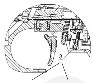
Turning screw 3 clockwise increases the second stage pressure
